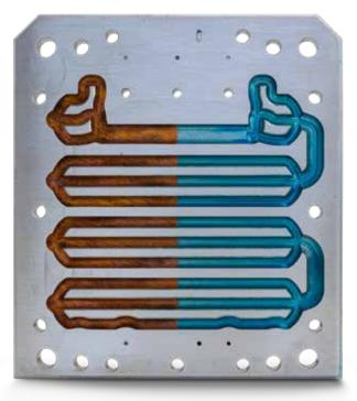
The function of a contour-following tempered tool insert depends on an unimpaired surface. That is why we now also offer our own channel coating as an option.
