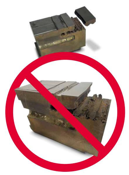
Here you can see severe corrosion damage that led to the breakage of the tool insert.
