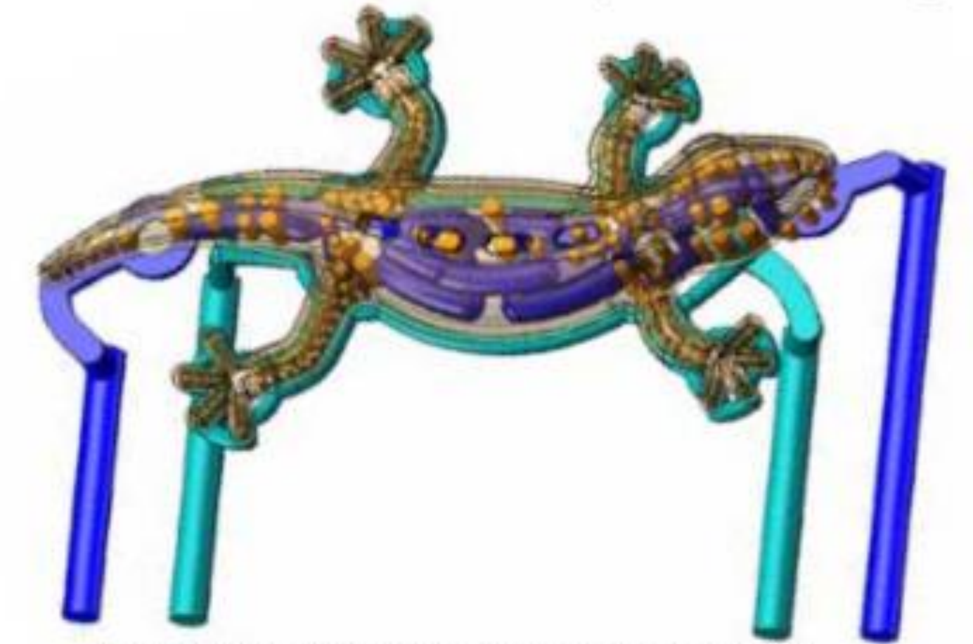
Contoured mold temperature control at the ejector side. Divided into two zones.
