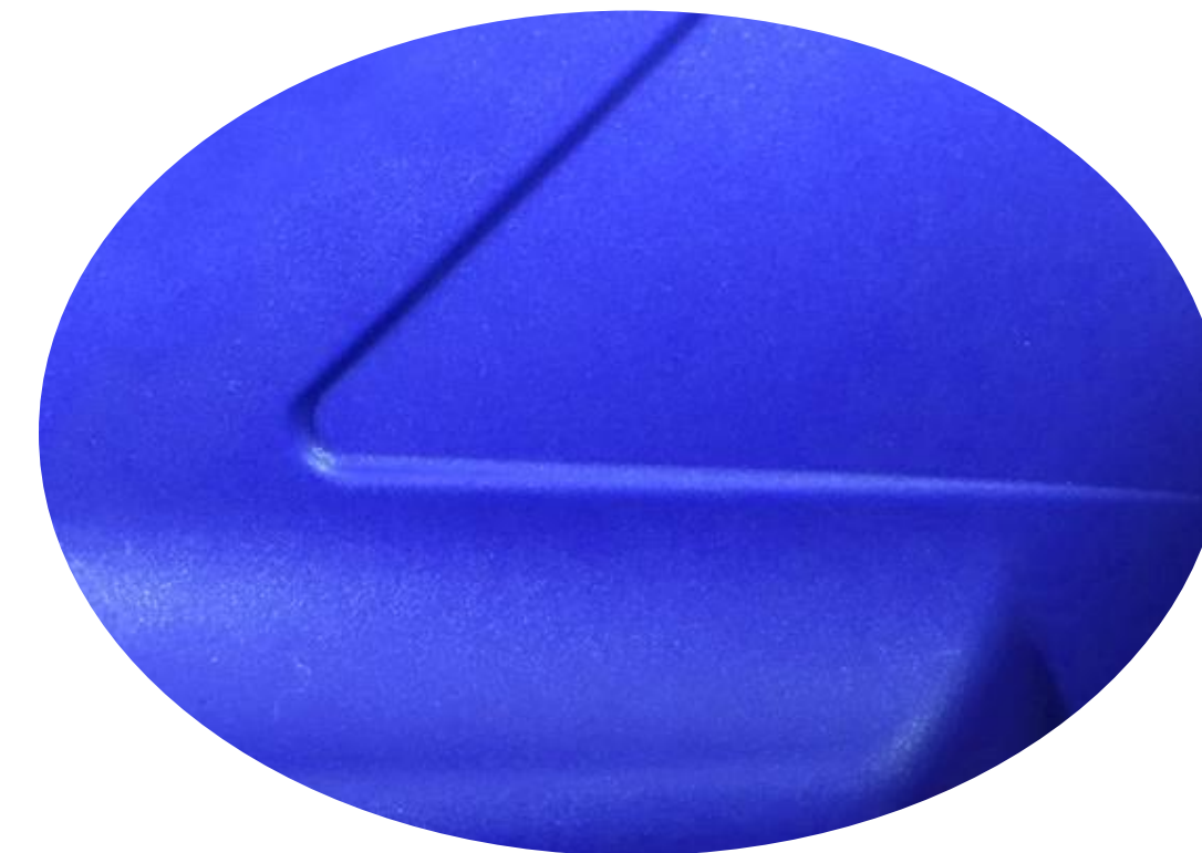
variothermal process 160°C injection 80°C during cooling
