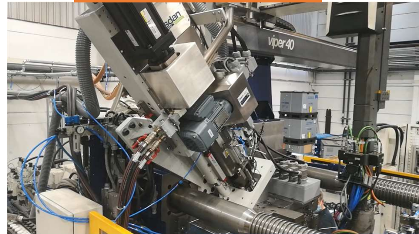
Angular application direct on tool and fixed plate face together with handling robot
