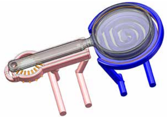
The variothermal, conformal tempering channels are located on the cavity half, divided into two zones.
