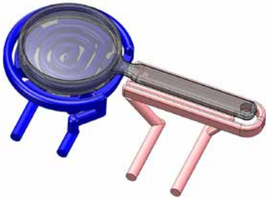
Contour-following tempering of the ejector half. Controllable in two different cycles.
