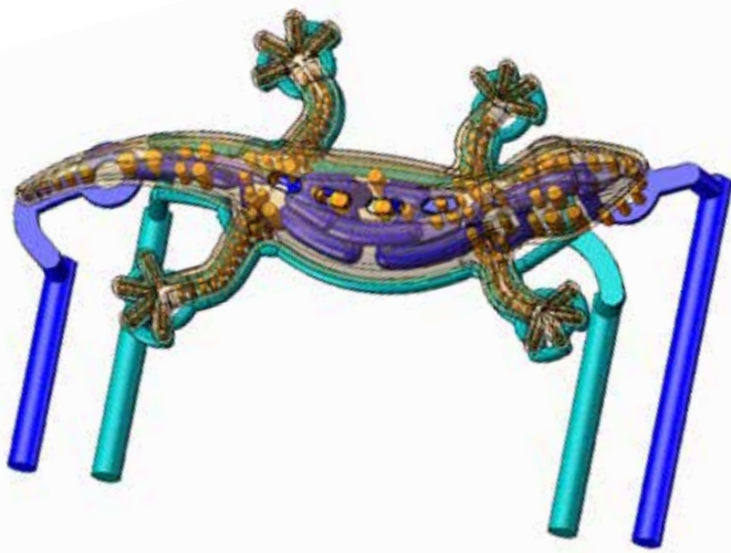
Contour-following temperature control on the injector side. Controllable in two different cycles.
