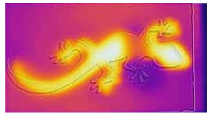
In the thermal image visible blockage of a cooling channel
